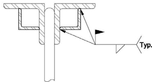
**Figure 3.4 Top Chord Reinforcement - Angles**
