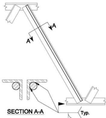
Figure 3.19 Rod Reinforcing
