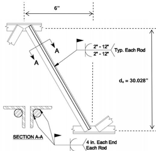
**Figure 3.41 Double Angle Reinforcing with Rod**
