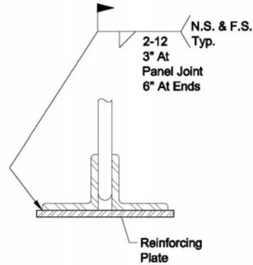
Figure 3.9 Bottom Chord Reinforcement
