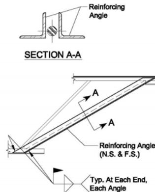
Figure 3.21 End Diagonal Reinforcing
