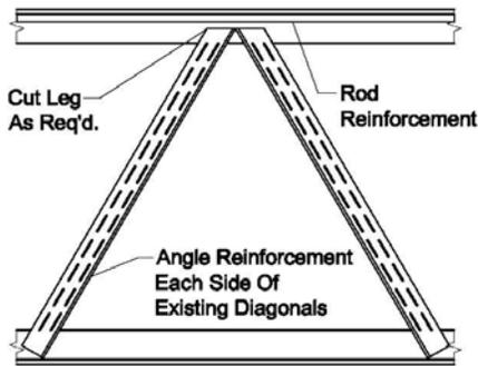
Figure 3.10 Angle Reinforcement on Rod Web Joist
