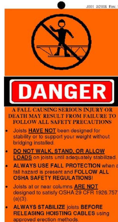
Figure 13 Typical joist manufacturer’s Danger Tag attached to every Column Joist
