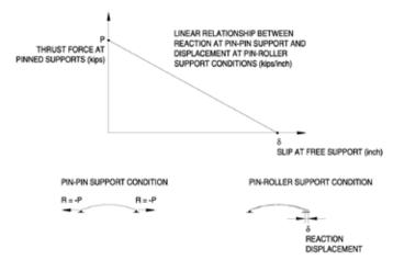
The new catalog includes text and illustrations providing guidance on design considerations such as load, span, seat depth, bridging, and horizontal deflection (shown here). graphic by: New Millennium Building Systems
