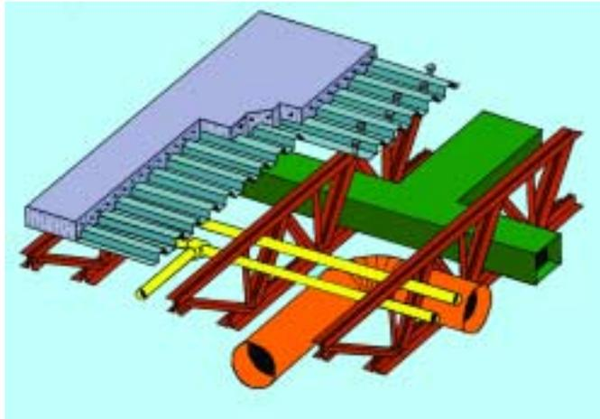
the 26-story 312 Elm Street building in Cincinnati. The lower 10 stories, covering 410,000 sq. ft, used cast-in-place concrete for the parking garage. Composite joists spanning 48.5' supported the upper 16 steel-framed office floors, which covered 326,000 sq. ft. The project had a 16-month construction schedule and \$60-million budget.
