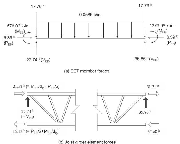
Fig. 7. Conversion of forces for 1.2D + 1.3W + 0.5S.
