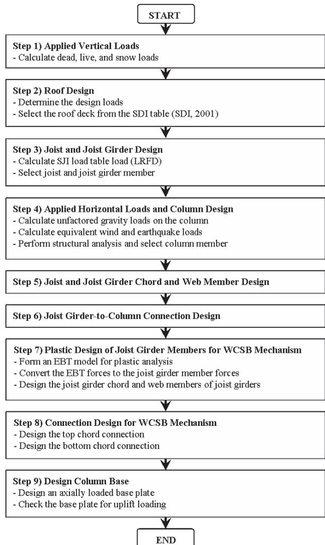
Fig. 2. Flowchart for proposed seismic design procedure.
