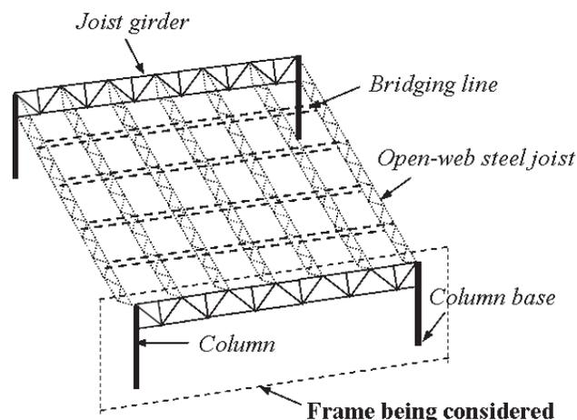
Fig. 1. One-bay, one-story steel joist girder structure.
