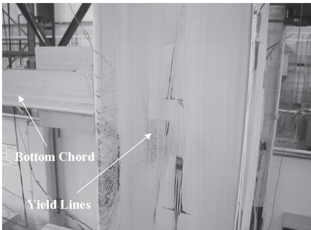
Fig. 11. Plastic hinge formation on the column.
