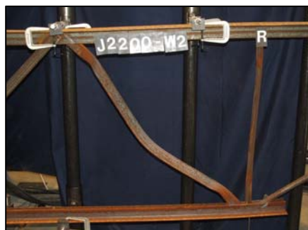
Figure 5 In-plane buckling of the uncrimped section (J2200-W2)
