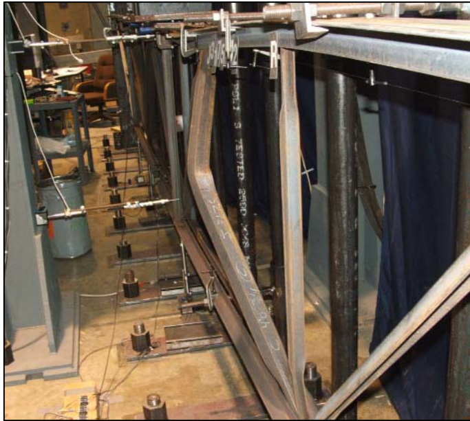
Figure 6 Out of plane buckling of the uncrimped section (J3175-W2)
