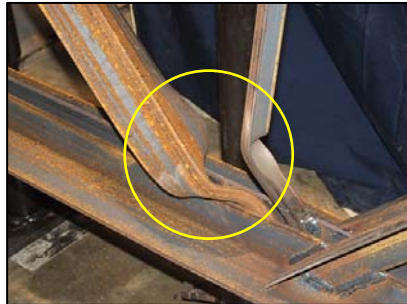
Figure 3 Out of plane buckling at the crimp (J3250-W1)
